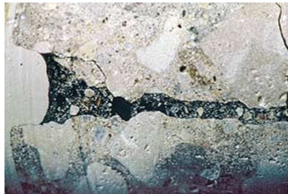
Fig. 23: Cores being taken after completion of injection
